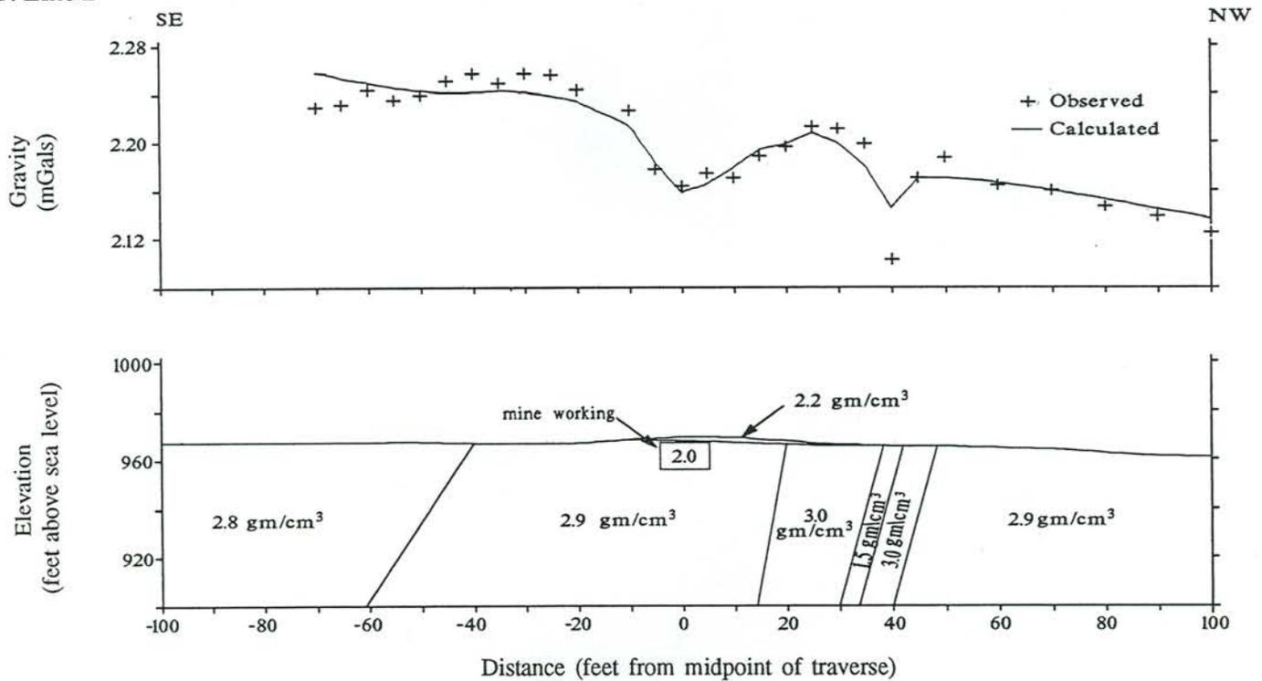
Figure 5. Gravity profiles for lines 1 and 2 showing observed gravity data with calculated data obtained from models.
