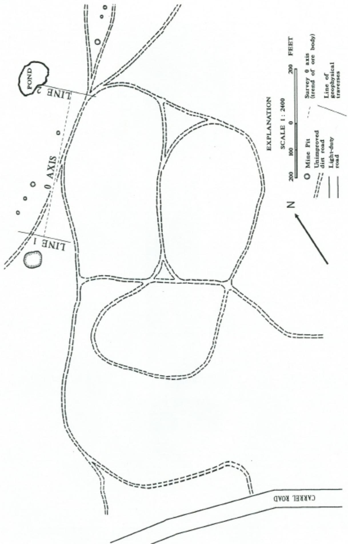
Figure 2. Site map of the abandoned Lawrence Iron Mine showing location of geophysical lines.
