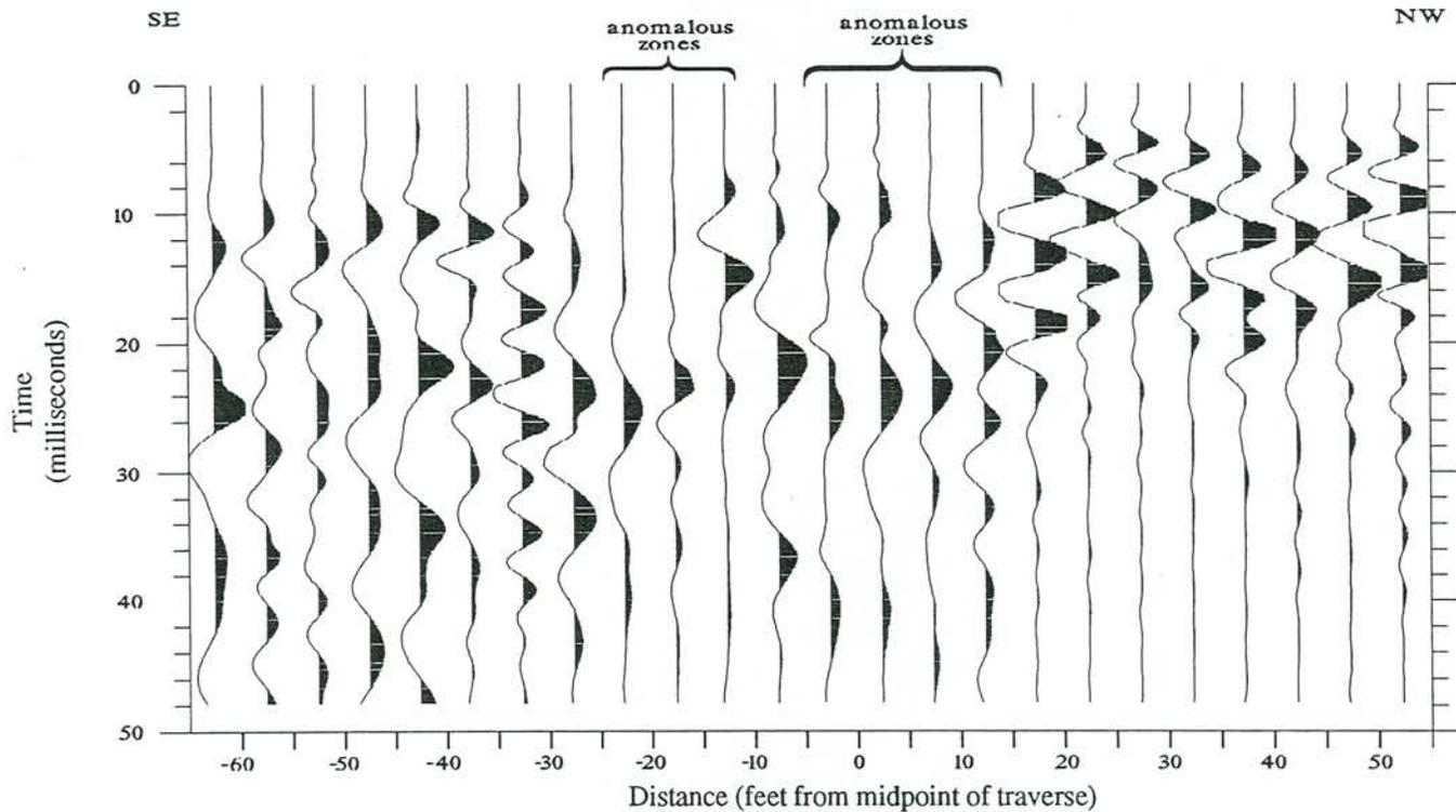
Figure 6. Common-offset reflection data for lines 1 and 2. Traces are positioned at midpoint locations between shotpoint and geophone. Anomalous zones are indicated by delayed first arrivals, and attenuated amplitudes.
