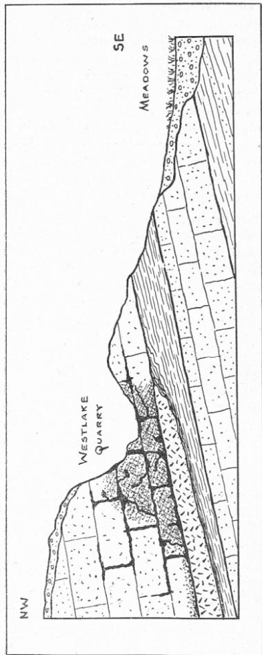
FIG. 5. Generalized cross-section at the old Westlake sandstone quarry, located about one mile southwest of the Schuyler mine. Copper ore was found in mineralized sandstone above the margin of the Arlington diabase sill, here about 6-10 feet thick. (After Darton.)
