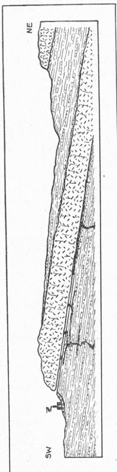
FIG. 7. Generalized cross-section at the American copper mine near Somerville, New Jersey. The main workings followed the under surface of the basaltic flow of First Watchung Mountain.
