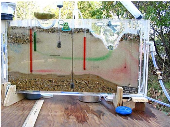
Figure 2. Plexiglas ground water model. Photo by S.W. Johnson
